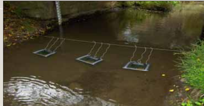
Figure 2. Stream bait survey in Dandenong Creek where 5 bait leaves are placed in each bag and floated in the creek for 1-3 weeks.
