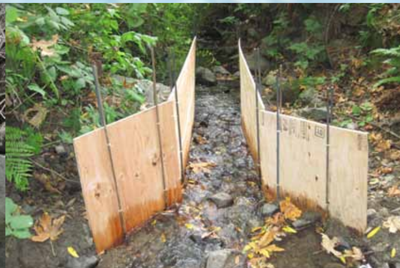
Left: Lisa Hunt, a Ph.D. student in Vince Resh's lab, surveys the quantities of aquatic insects in Strawberry Creek. Right: Researchers on the Strawberry Creek project built reinforcements to test the effects of augmenting water flow.
